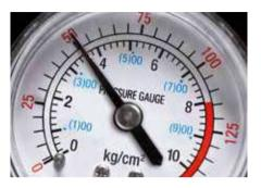
An air-pressure gauge shows exactly if the tyres are at the right pressure.
