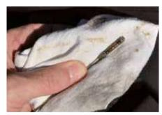
You check the oil level with a clean lint-free cloth. There is a minimum and maximum mark on the bottom of the dip stick.
