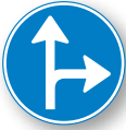
D6 Instruction to follow one of the directions ahead shown by the arrows.
